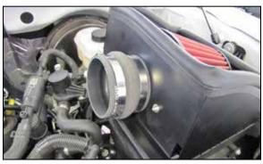
12. Install the provided hump coupler (08699) onto the filter adapter and secure with the provided hose clamp.
