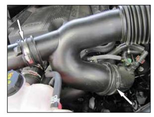
5. Loosen the two hose clamps that secure the factory intake tube to the turbo inlets and remove the factory tube from the vehicle.
