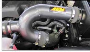
17. Install the AEM® intake tube into the couplers at the turbo inlet tubes and then into the coupler at the filter adapter, adjust the tubes for best fit and then secure with the provided hose clamps.
