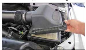
4. Release the locking clips that secure the upper air filter housing to the lower housing, then lift the upper housing and remove it from the vehicle. Remove the factory air filter from the vehicle. NOTE: AEM recommends that customers do not discard factory air intake.
