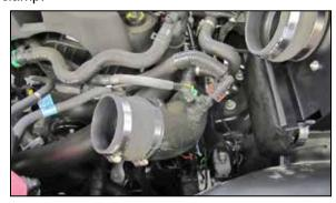
13. Install the provided coupler (08497) onto the driver's side turbo inlet tube and secure with the provided hose clamp.
